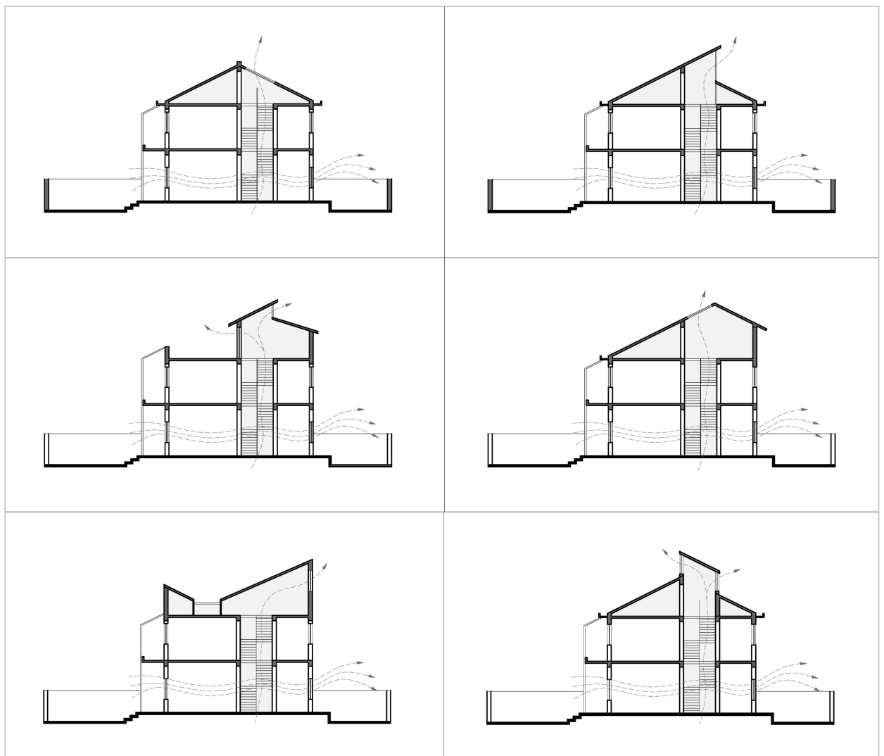
Fig.5-7 Vertical draft and roof space
