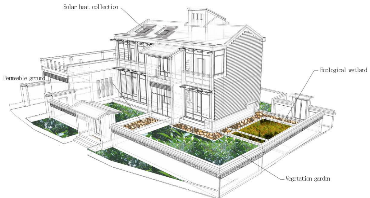
Fig. 6-25. Integrated technologies in renovation
